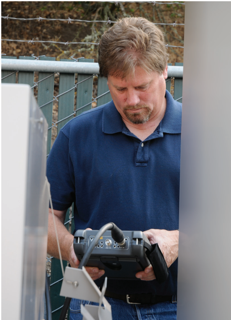
View and control the return loss and DTF displays independently
