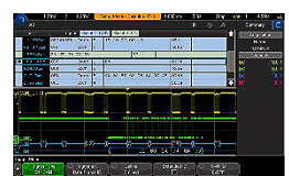
Figure 19: Multi-bus time aligned decode.
