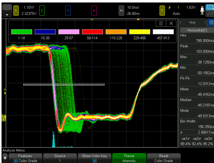
Figure 15. Color grade and histogram on a jittery clock edge.
